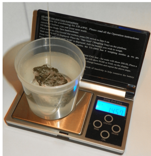
Figure 1.19 - Rapid measurement of sample volume by freely suspending and submersing specimen in a water-filled and tared plastic container. Balance readout is equivalent to volume of object in \text{cm}^3 .
