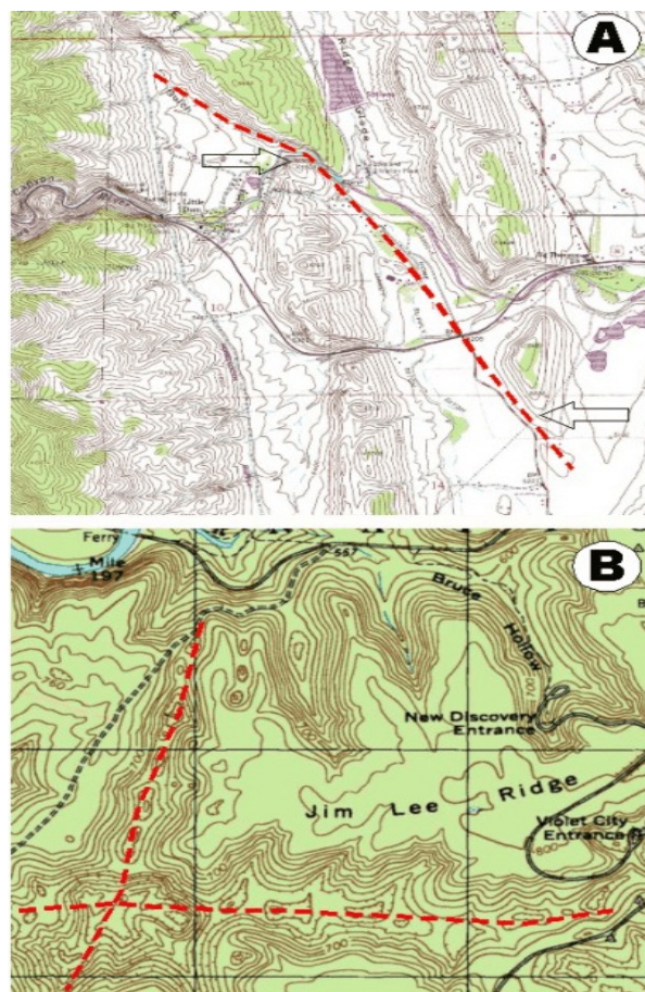
Figure 11.3 - Examples of fault identification from topographic maps.
